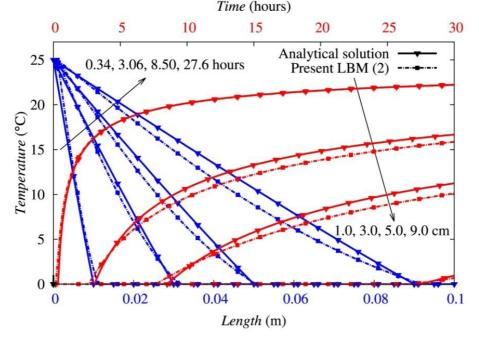
*Figure 3. Temperature profiles at different times and at different positions: blue lines for the temperature distributions at times and red lines for the temperature distributions at positions.*
