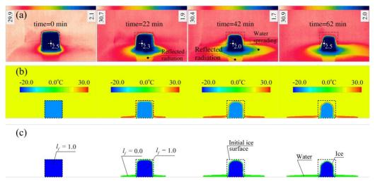
Figure 4. Time sequences of the experimental and numerical results for an ice cube melting in ambient air. (a) Infrared images of the ice cube and ambient condition; (b) numerically determined temperature field; (c) numerically determined ice and water phases.
