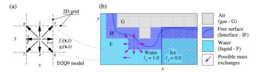
*Figure 1. General scheme of the proposed model. (a) D2Q9 lattice configuration on the 2D grid; (b) materials in the domain and free surface representation.*
