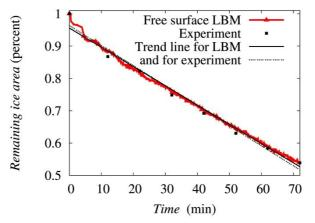
Figure 5. Experimentally and numerically determined remaining ice area.
