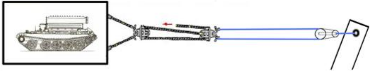
Figure 7. Pulley System of a Single BTS-4 Model Tractor
