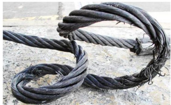
Figure 9. Broken steel wire ropes
